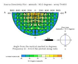
When comparing the two radiation plots it can be seen that there is more high frequency energy emitted side-ways from the array than from front-to-back.
