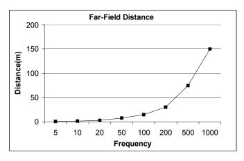
The higher the frequency the greater the distance from the array before the sound appears to be coming from a point source.
