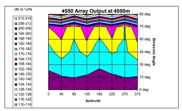
At a distance of 4000m, the 183 dB isopleth occurs at emission angles less than 25 degrees. Along the horizontal, the amplitudes are very small, less than 120 dB.
