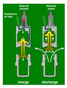
For each airgun, the amplitude (or loudness) of the seismic signal is a function of the volume and pressure of the air inside the cylinder and the cylinder's depth under the water surface. As with a balloon, the larger the cylinder volume and the higher the internal air pressure, the louder the "pop".
