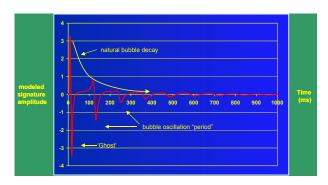
This signature shows the first, or primary, positive pressure pulse due to the initial expansion of the bubble. The following negative pulse, referred to as the "ghost", is due to the reflection of the initial pulse at
