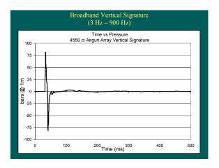
For the purpose of evaluating the environmental impact of an airgun source, the signature should be reported at the widest practical bandwidth. Therefore, the following plots show the time signature and amplitude spectrum for a typical airgun array in the 3 – 900 Hz frequency band.
