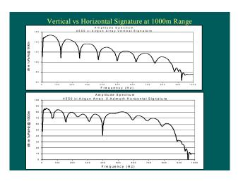
Notice the difference in the amplitude scales between the vertical and horizontal signatures. The amplitude of the horizontal signature is almost 60 dB below (or 1/1000) that of the vertical signature.
