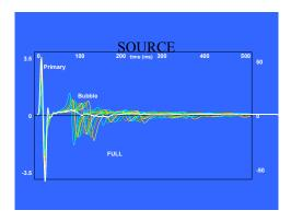
It is common in the seismic industry to quote the output of a particular airgun array in terms of time vs pressure (time domain signature) and frequency content characteristics. The time domain parameters quantify certain characteristics of the source signature.
