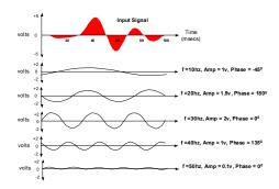
As shown, the signal at the top is composed of five discrete frequencies: 10, 20, 30, 40, and 50 Hz. Each frequency component has an associated strength (amplitude). When the amplitude values are plotted as a function of frequency, the signal's amplitude spectrum is produced.
